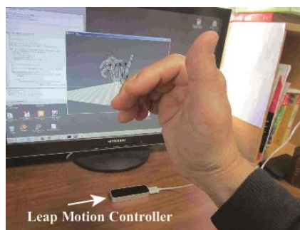
Figure 7: Digital hand system with LMC to get hand posture in real time.
